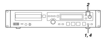
After entering record-ready mode (→ p.25), press the SYNC REC button repeatedly to select "Sync ALL" or "Sync 1".
